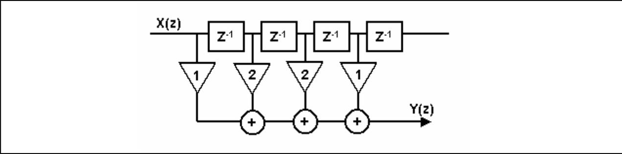
Figure 2. Schematic of a Four Element FIR Filter
