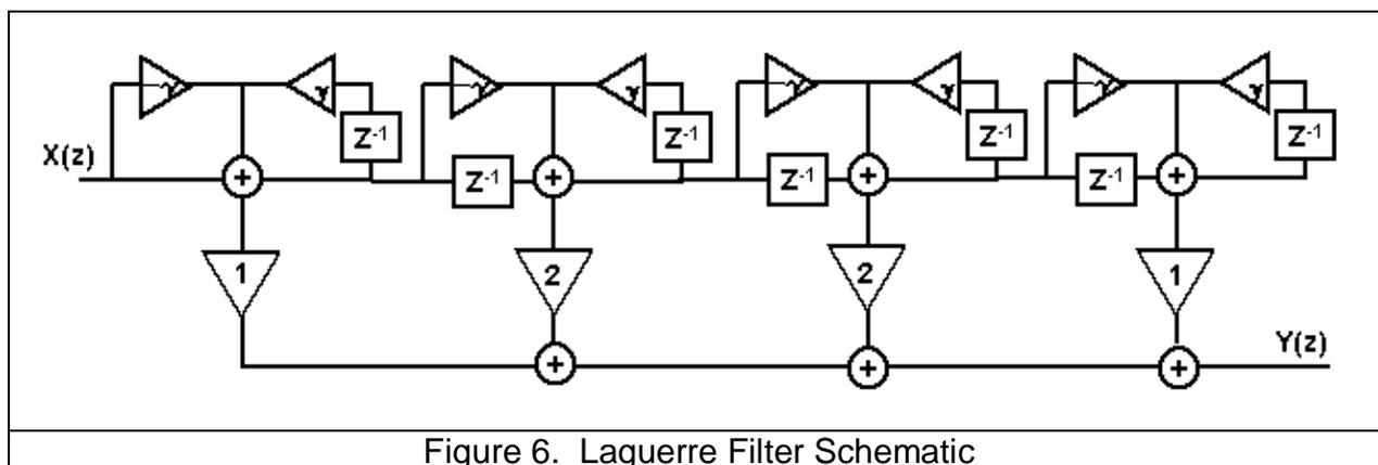
The EasyLanguage code for a four element Laguerre Filter is given in Figure 7. L0 is the output of the first section, and is just an EMA. The following three sections are identical in their form. The four sections of the Laguerre delay line are summed exactly the same way as one would sum a linear delay line for a FIR filter. The Laguerre output is the "Filt" variable. An identical length FIR filter is also computed for comparison.
