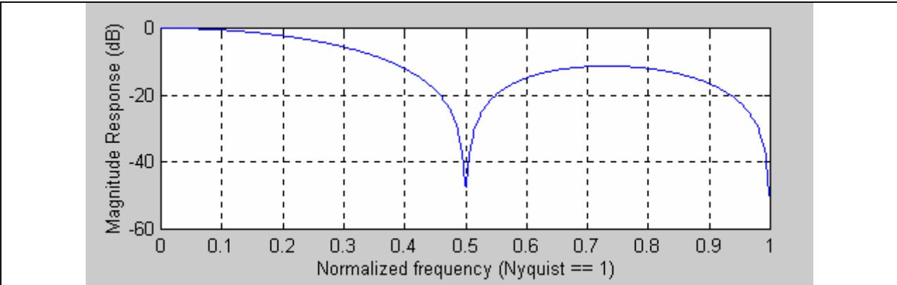
Figure 3. Four Bar Moving Average Frequency Response
