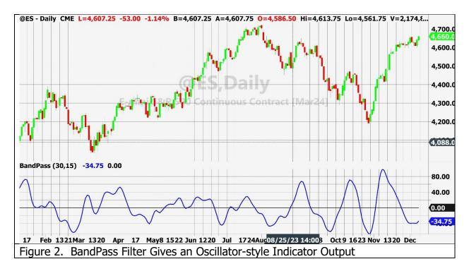
This BandPass filter is superior to a second order BandPass filter because it provides sharper transitions between the pass band and the stop bands. Think of it this way: The second order BandPass applies one order to the upper filter edge and one order to the lower filter edge, whereas this BandPass filter applies two orders to both the upper and lower band edges.
